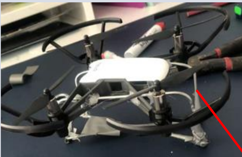
Figure a: Drone with the DIY payloads dropper glued on it
