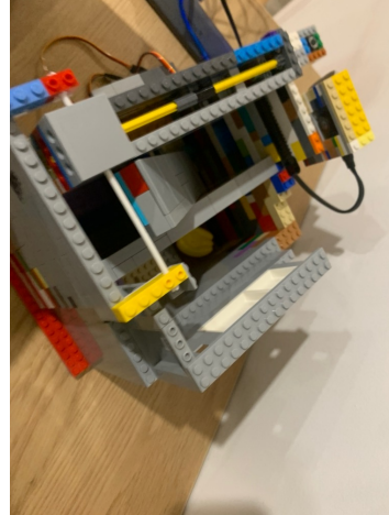
The platform tilts and the bottle falls into the recycling bin
