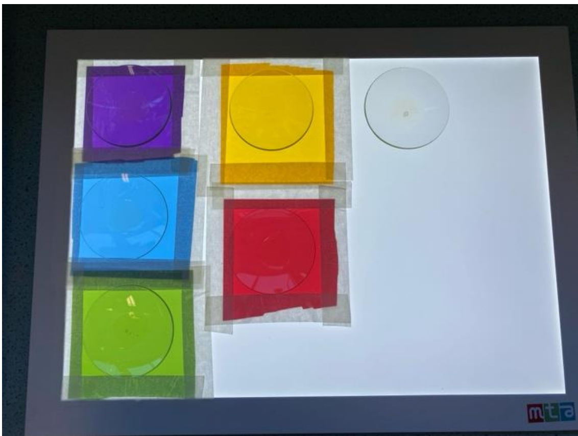
Figure 3: Experimental setup of light treatment. Staphylococcus epidermidis samples were treated using a 240V backlit MTA light panel (KD1022). Colour was changed using 5 different coloured filters: red, yellow, green, blue and violet. A control sample was treated with unfiltered white light. Samples were placed on a watch glass during treatment.
