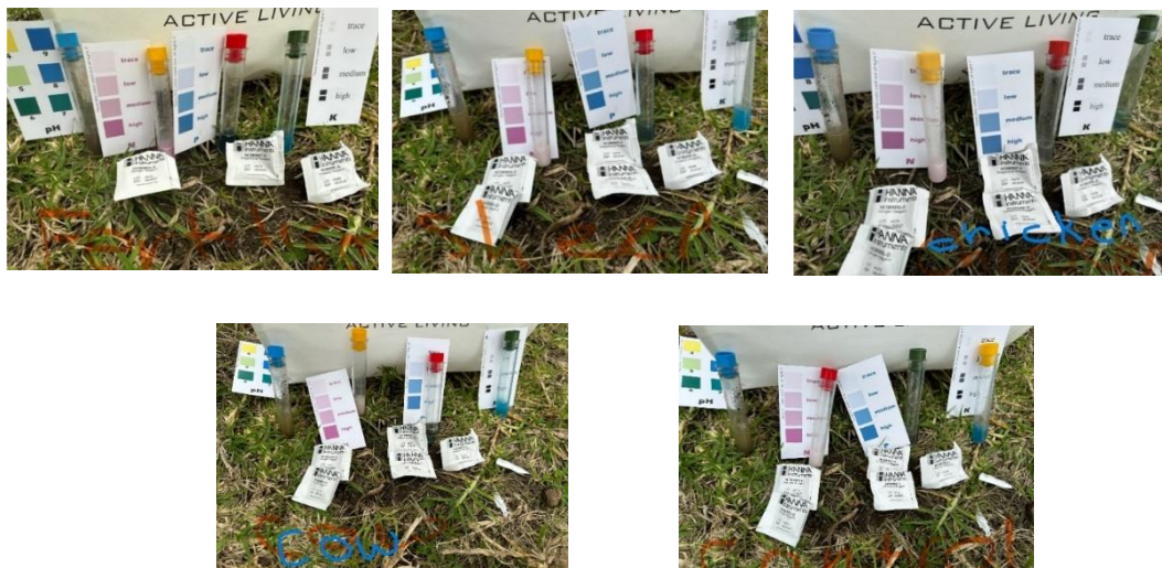
Figure 3 Soil pH testing soil L-R top commercial fertiliser, sheep, chicken; L-R bottom- cow control
