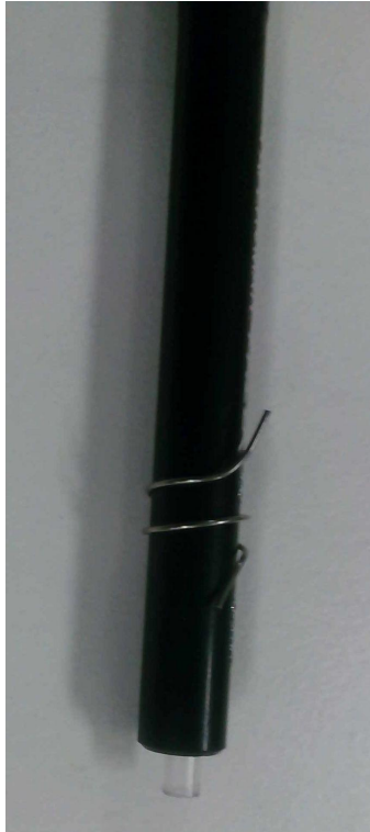
A picture of the first length of nichrome wire wound around the pacer pencil .
