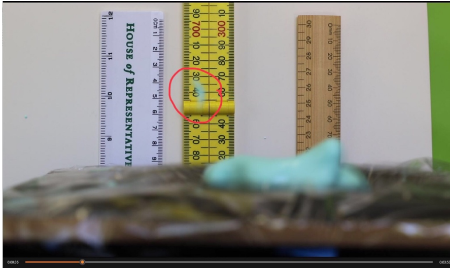
Figure 11 Example of small drops shooting off at much higher levels
