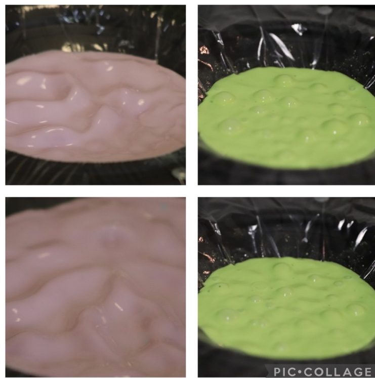
Figure 5 40Hz Sawtooth created ripple and bubble effects in the oobleck
