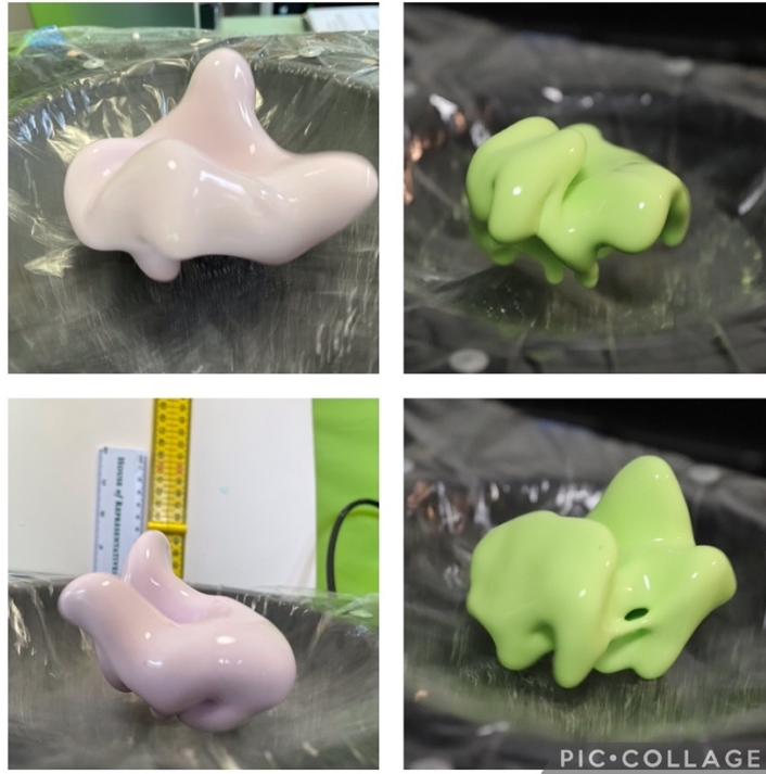
Figure 6 40 Hz Sine became a single very active ball of oobleck
