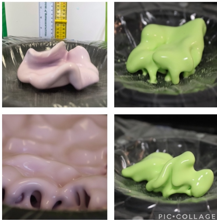
Figure 7 40Hz Square took longer to form a single mass and bounced lower in the speaker
