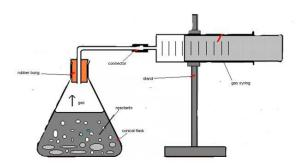
Figure. Basic experiment set up to collect oxygen gas
