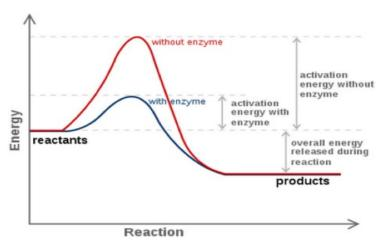
**Figure 1.** Differences in activation energy between reactions with and without enzyme Reference: https://www2.nau.edu/lrm22/lessons/enzymes/enzymes.html
