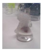
Figure. Overflowing of oxygen gas for pH 3 solution.
