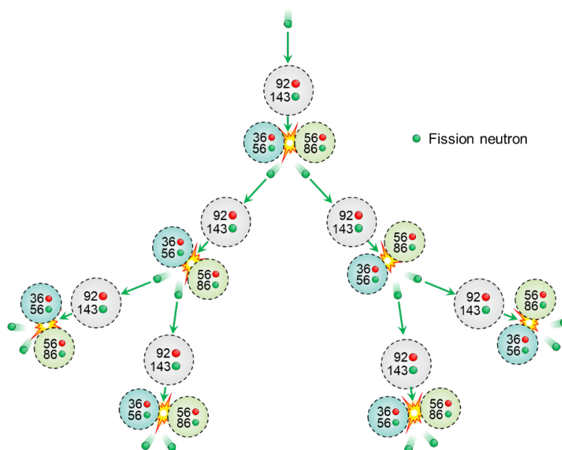
Figure 6.37: Nuclear chain reaction
