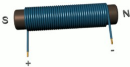
Diagram 3: Solenoid with copper wire.
