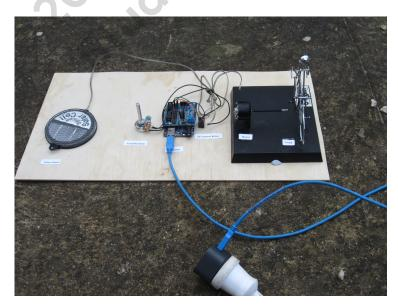
You also need a strong light to simulate the sun (or use the sun). I used the sun and slowly moved a piece of cardboard across the solar panel to simulate sunlight coming and going. I could hear the click of the relay and saw the bike pedals immediately moving. If the sun is not strong enough (behind a cloud), you can use a strong light. I could do this using a spot light.
