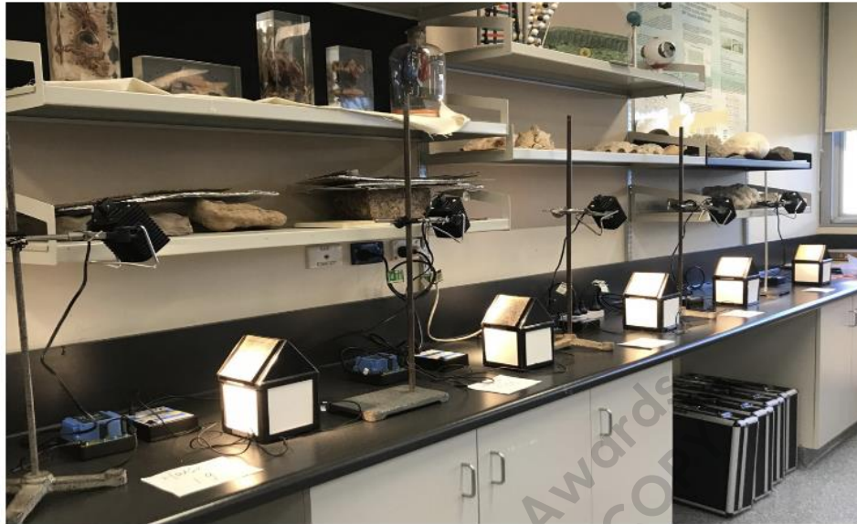
Figure 4: The internal temperature testing of all five houses with different amounts of black carbon deposits (0.00g, 0.25g, 0.50g, 0.75g, 1.00g) on roofing materials (cardboards)
