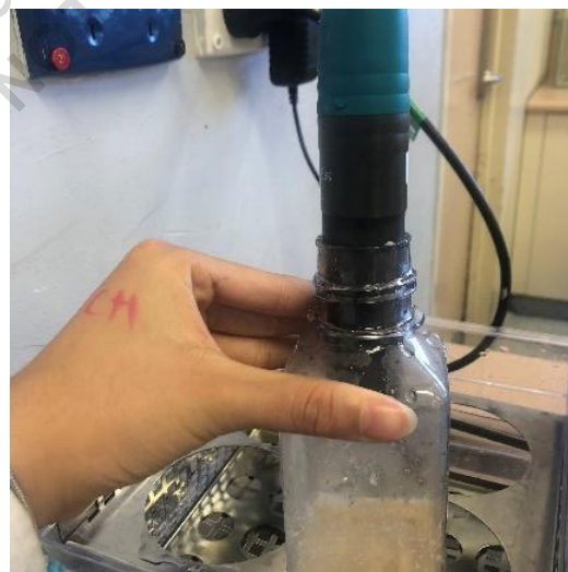
Figure 2 – Positioning of the Vernier carbon dioxide gas probe inside the experimental bottle
