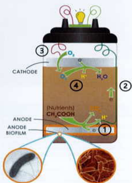
Figure 1. shows the flow of electrons through a single-chamber MFC.
