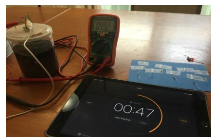
5. Connecting the multimeter's leads on the wire ends of the resistor (leave the resistor plugged in for 2 minutes).
