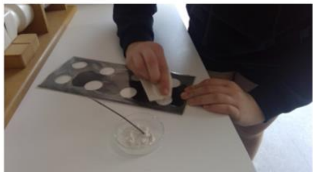
Figure 6: Spreading the sunscreen on the testing circle template with the paper towel.
