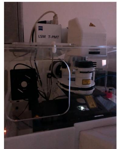
Figure 24: The confocal LSM 700 microscope that was used to view the live/dead bacterial biofilms
