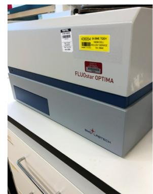
Figure 23: The FLUOstar microplate reader with fluorescent light
