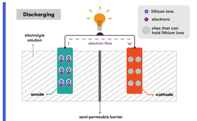
An illustration of a lithium-ion battery during discharge. *Source:* <https://www.science.org.au/curious/technology-future/lithium-ion-batteries>
