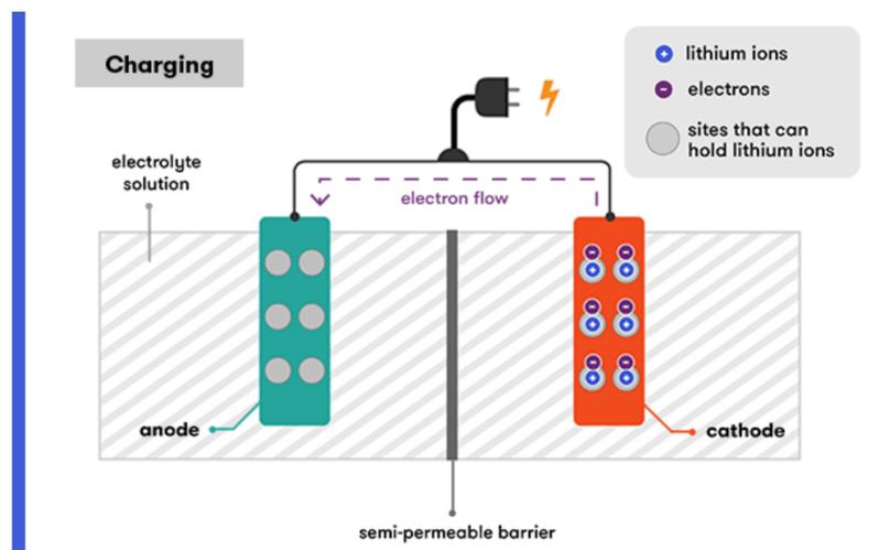
An illustration of a lithium-ion battery while charging. *Source:* <https://www.science.org.au/curious/technology-future/lithium-ion-batteries>
